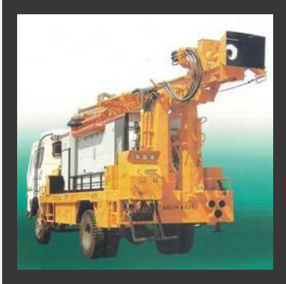
Truck Mounted Drill Rig
