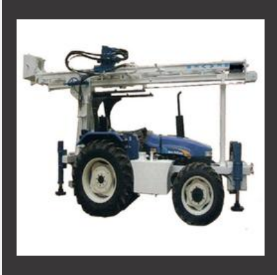
Tractor Mounted Water Well Drill Rig
