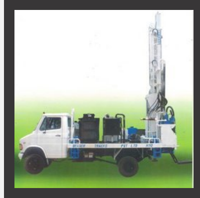
Pickup Mounted Water Well Drill Rig
