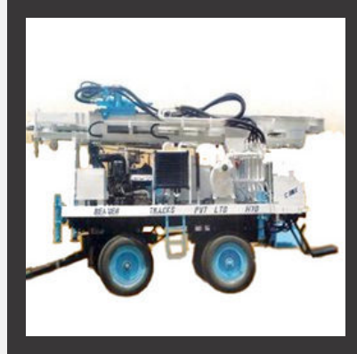
Drilling Rig Mounted On Trailer
