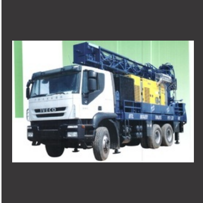
Heavy Duty Water Well Drilling Rig
