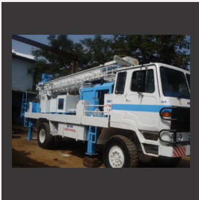
Rotary DTH Drill Rig
