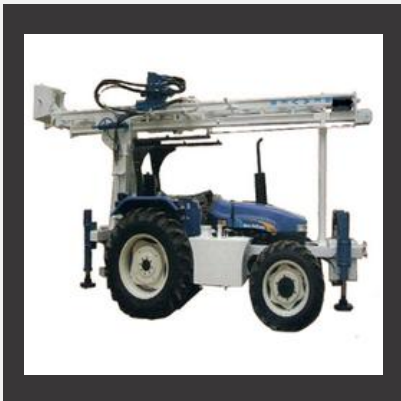
Tractor Mounted Core Drilling Rig
